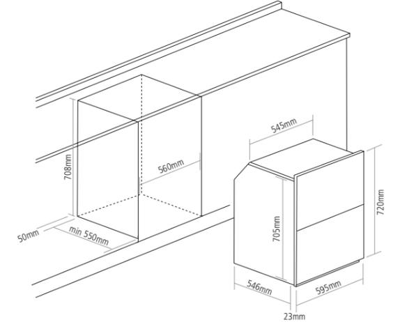
We recommend that when installing a stack or quad of products, a pair of our installation brackets [OVEN/BRACKETS2] are purchased to support the upper product ensuring a seamless fit for each appliance when one is on top of the other.
