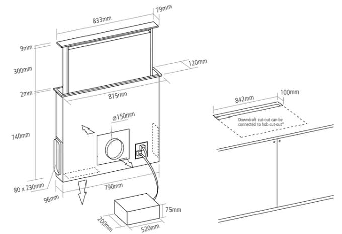
\*For electric hobs only. A 50mm gap is required for gas hobs.
