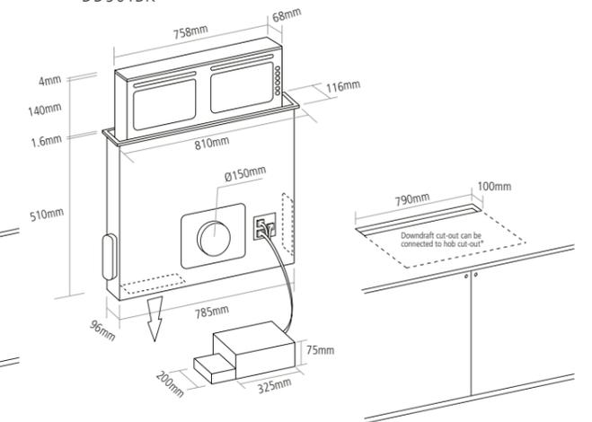
\*For electric hobs only. A 50mm gap is required for gas hobs.
