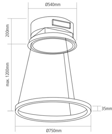
For installation create a false ceiling with a round niche of 510mm, with a minimum height of 220mm.
