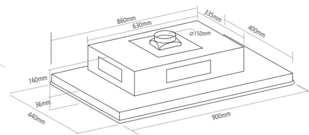
For installation into the ceiling a niche of 815mm x 515mm is required, with a minimum height of 170mm
