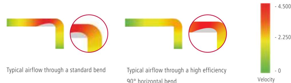
Typical airflow through a standard bend
